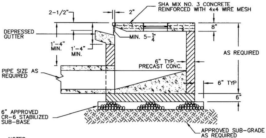
1. CHANNEL SHALL BE BRICK OR HAND FORMED CONCRETE MIN. THICKNESS OF 4".
